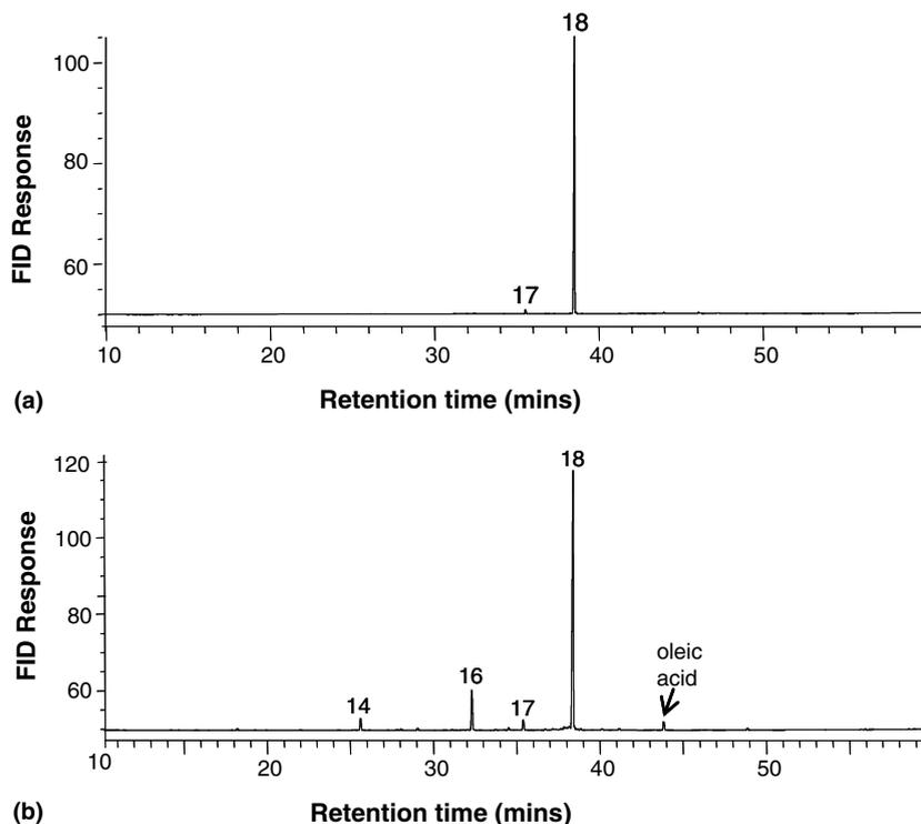
Fig. 4. GC–FID traces showing the total product distributions obtained from HyPy of fatty acid model compounds, (a) stearic acid and (b) oleic acid, which had been pre-adsorbed on silica gel. (Numbers refer to carbon chain lengths of *n*-alkane products.) Taken from Craig et al., 2004 (reproduced with permission).
