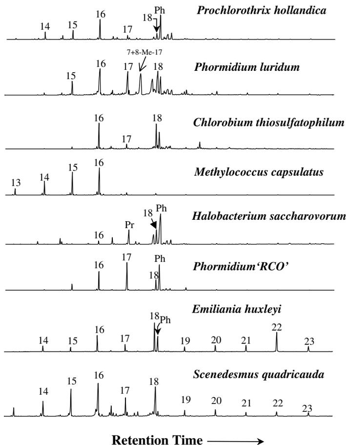
Fig. 3. Partial  $m/z$  85 ion chromatogram showing the distribution of  $n$ -alkanes and isoprenoids in the  $C_{13}$ – $C_{23}$  carbon number range produced from HyPy of a selection of unextracted microbial cultures. (Numbers refer to carbon chain lengths of  $n$ -alkane products; Ph = phytane.)
