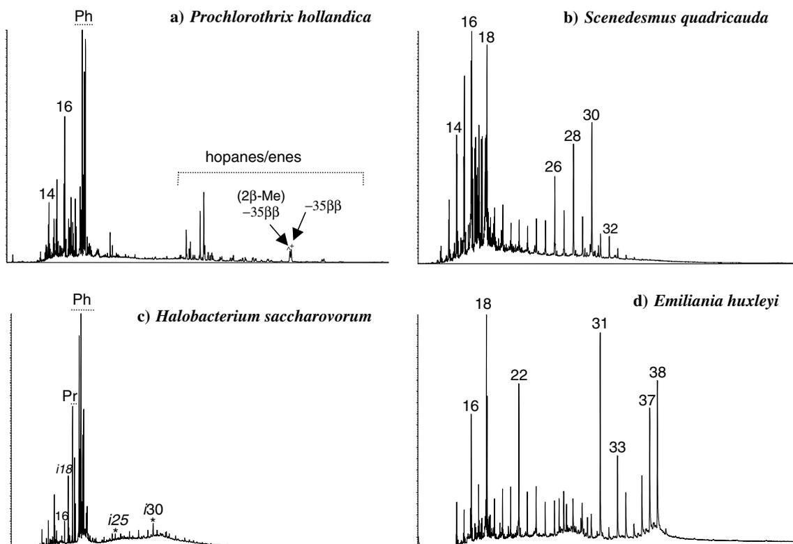
Fig. 1. Total ion chromatograms (TICs) showing the aliphatic hydrocarbon product distributions generated from HyPy of unextracted cells of (a) *P. hollandica*, (b) *S. quadricauda*, (c) *H. saccharovorum*, and (d) *E. huxleyi* (grown at 10 °C). (Numbers refer to carbon chain lengths of *n*-alkane products; Ph = phytane + phytene; Pr = pristane + pristene; *i*18, *i*25 and *i*30 = C<sub>18</sub>, C<sub>25</sub> and C<sub>30</sub> regular isoprenoids.)
