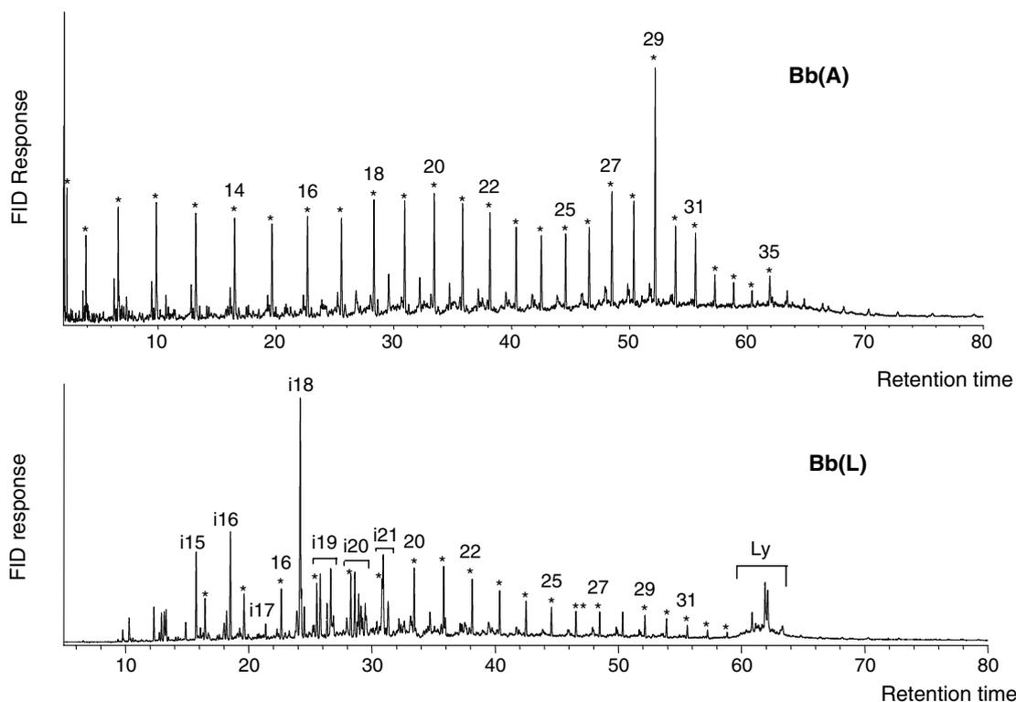
Fig. 7. GC–FID profiles of total products generated from HyPy of algaenans of *B. braunii* races A [Bb(A)] and L [Bb(L)]. (Numbers refer to carbon chain lengths of *n*-alkane products; *i* denotes isoprenoids; Ly = lycopane, lycopenes and monoaromatic  $C_{40}$ .)
