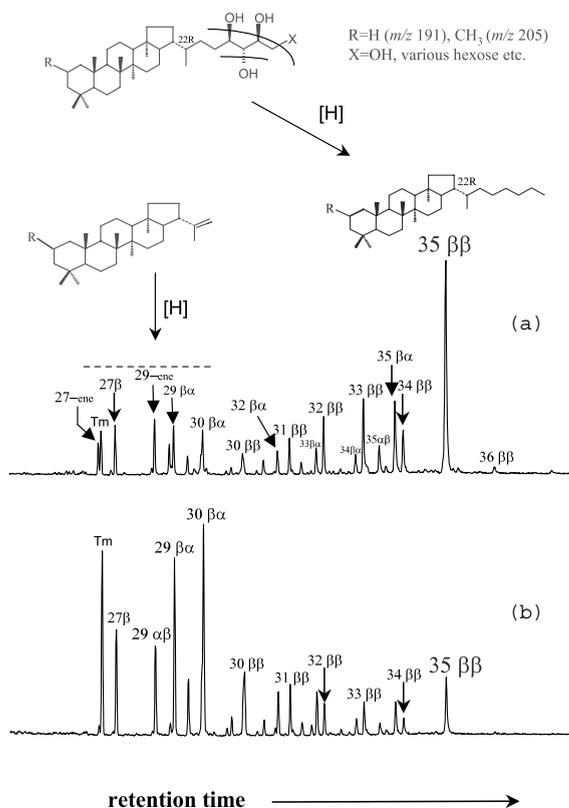
Fig. 5. *m/z* 191 ion chromatograms showing the distributions of hopanes produced from HyPy of *P. luridum* (cyanobacterium) whole cells using (a) the optimised HyPy procedure with a Mo catalyst, and (b) HyPy without a Mo catalyst.
