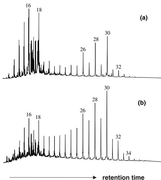
Fig. 6. Total ion chromatograms (TICs) showing the distributions of aliphatic hydrocarbons generated from HyPy of (a) unextracted, and (b) extracted cells of the freshwater chlorophyte *S. quadricauda*. (Numbers refer to carbon chain lengths of *n*-alkane products.)
