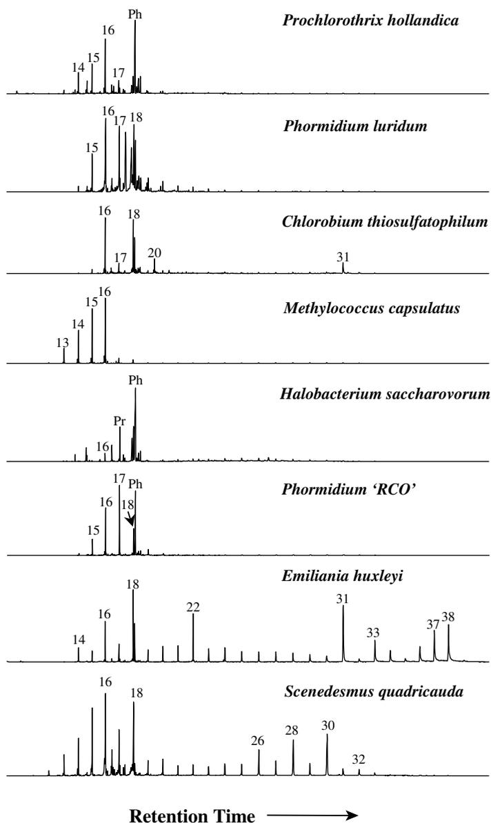
Fig. 2.  $m/z$  85 ion chromatograms showing the full distribution of  $n$ -alkanes and isoprenoids generated from HyPy of a selection of unextracted microbial cultures. (Numbers refer to carbon chain lengths of  $n$ -alkane products; Ph = phytane.)
