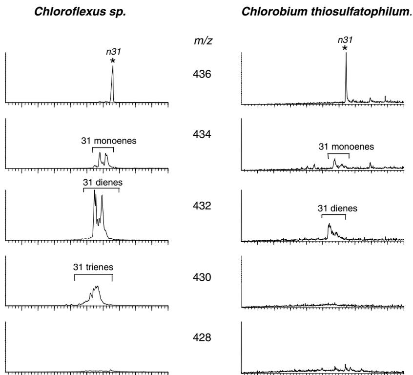
Fig. 10. Distribution of  $n$ - $C_{31}$  alkanes and alkenes generated from HyPy of *C. aurantiacus* and *Chlorobium thiosulfatophilum*, using the relative abundances of molecular ions detected by GC–MS.
